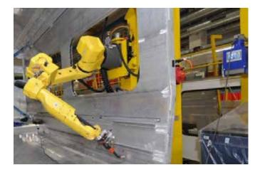
The robots are mounted on a platform, which is in turn sitting on a travel rail. Thus, the entire length of the vehicle body remains accessible. All chassis and travel axes are driven by high-precision steering racks and FANUC servomotors, which are easily integrated into the robot control as axes.
